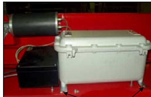
Fig. 13.2 shows an controller fixed on the roof of the car
